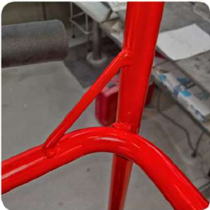
SAFETY HARNESS CONNECTOR POINTS EN 280/2013 3kN FORCE
