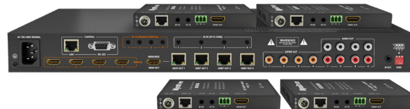
4x4 4K HDR HDBaseT Matrix Kit with HDCP 2.2, Audio Breakout and 4x PoH Receivers (4K: 35m/115ft | 1080p: 70m/230ft)
