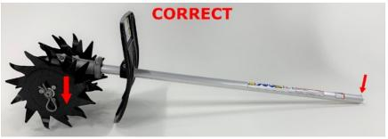
a box or assembled by the consumer. The recalled mini-cultivator attachments are those with the gearbox installed upside down.
