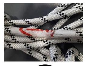
The recalled safety ropes have the model name and serial number on the label affixed to each end of the rope. Consumers should immediately stop using the recalled ropes and inspect the rope for a deep cut or tape connecting two ends of rope together, and if either is found, contact Petzl America for instructions on receiving a free replacement rope.
