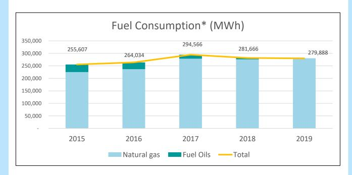
\*Since 2012 when we installed a natural gas feed system and TRT has since utilized natural gas as its primary fuel. We have the ability to also use #6 Oil, #2Oil and biofuels that we produce on site as a means to produce steam and electricity. The change to natural gas has had multiple positive effects. We now operate at a lower cost, more reliably and have lower overall emissions.
