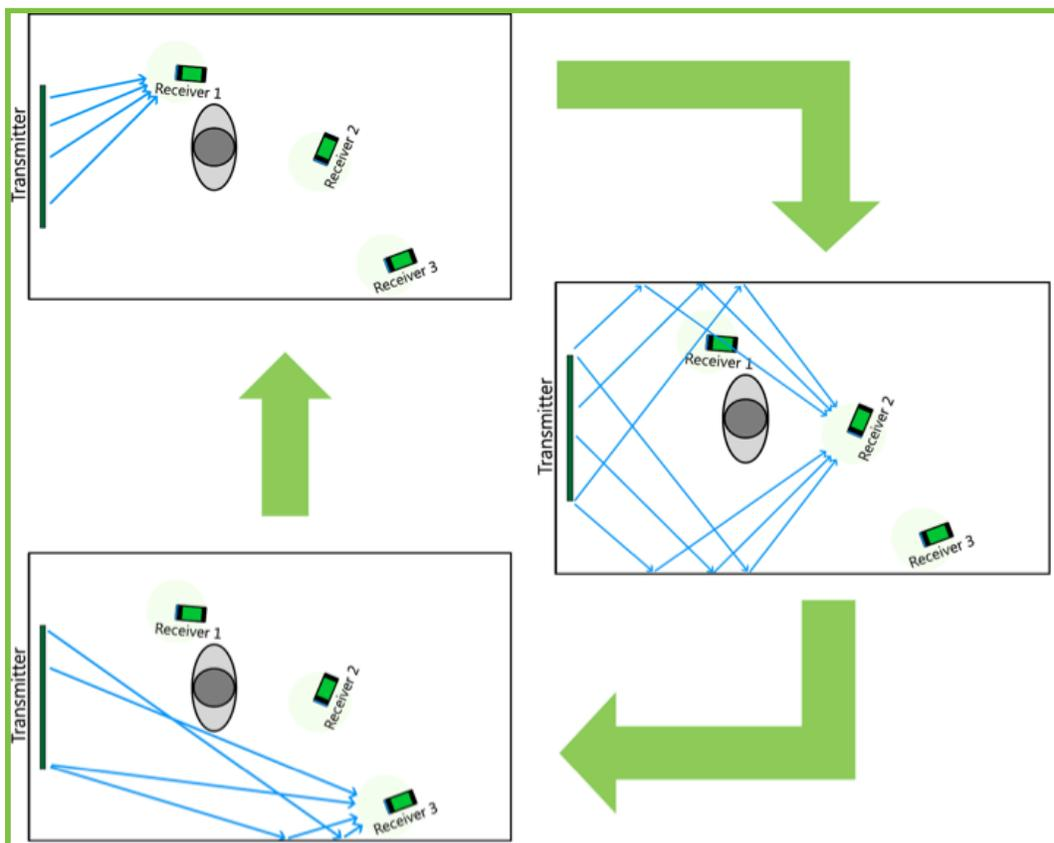
Cota is comparable to Wi-Fi or Bluetooth—the signals reflect off walls, ceilings and floors to find multiple paths between the transmitter and receiver. It's not only the most efficient way to send signals between a device and a power source, but also it's the safest.
