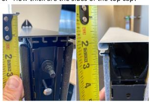
Insert Top Cap Side Thickness Measurement:
