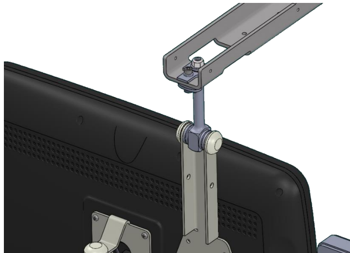
FIGURE 5B. MOUNTING DUAL ARM TO SWING ARM
