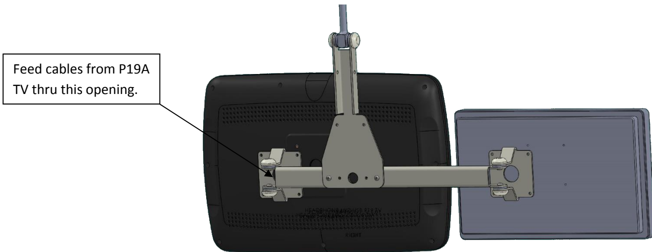
FIGURE 3. CONNECTING THE DUAL MOUNT ARM
