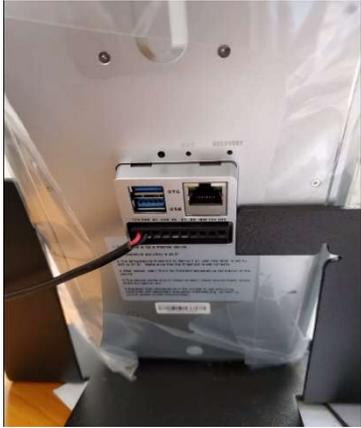
Connect the 10-position phoenix connector to the back of the PDI-TK8 unit (**Note:** the red power and black ground wires are on the left side of the unit as you're looking at the back of the unit). Next, plug the unit into the wall receptacle for power.
