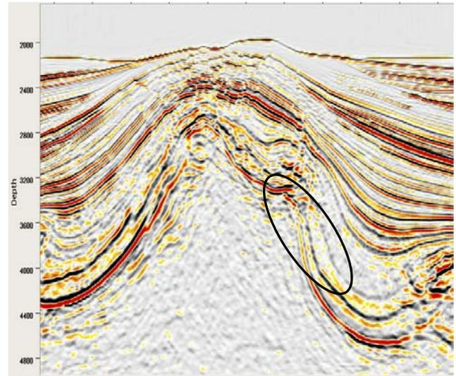
Figure 5: A PSDM stack migrated with a model updated without (top) and with structurally constrained tomography. The oval highlights the improved continuity.
