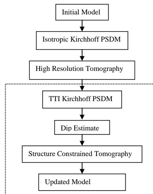
Figure 1: Workflow used for velocity model building with structurally constrained tomography. The dashed box shows processes iterated to obtain the best model.
