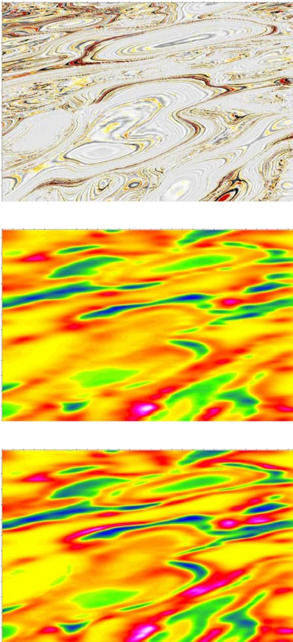
Figure 3: Depth slices from 3D seismic volume showing mini-basins(top), grid-based (middle) and structurally constrained (bottom) tomography updates. Structurally constrained updates follow the mini-basins outline.
