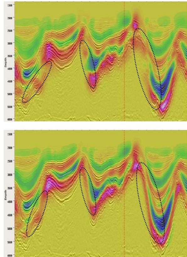
Figure 2: Migrated stack with tomography update overlay without (top) and with structural constrain. The main improvement occurs at basins flank.
