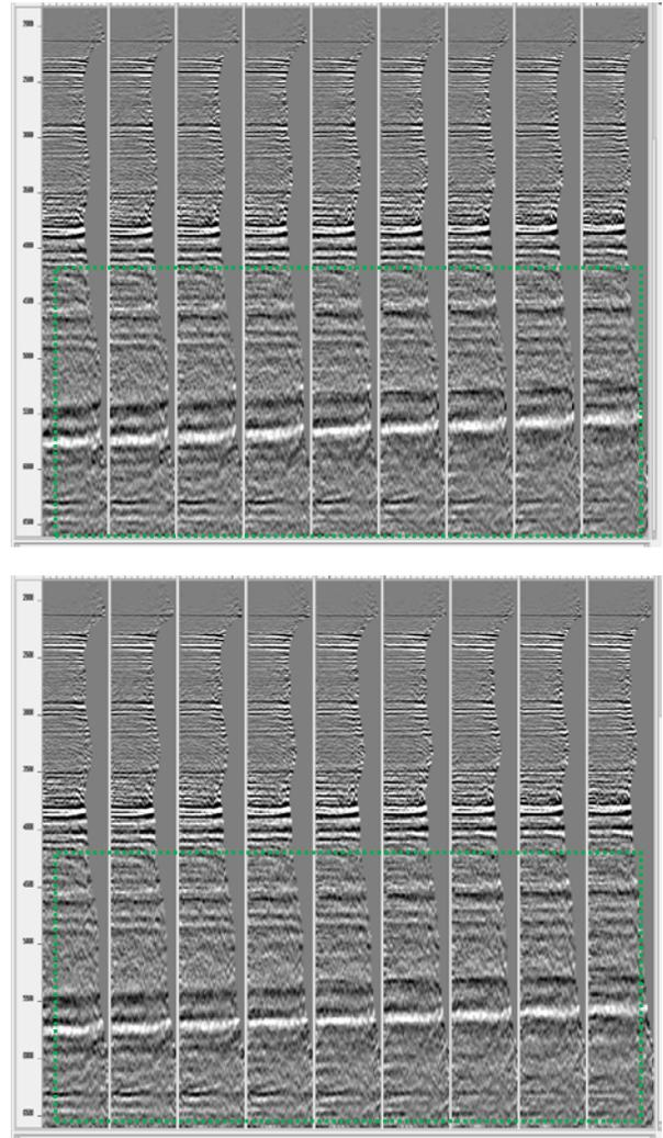
Figure 4: Gathers migrated using the model updated with grid-based tomography (top) and the ones with structurally constrained tomography. The bottom gathers show improved flatness below 4000 m depth.
