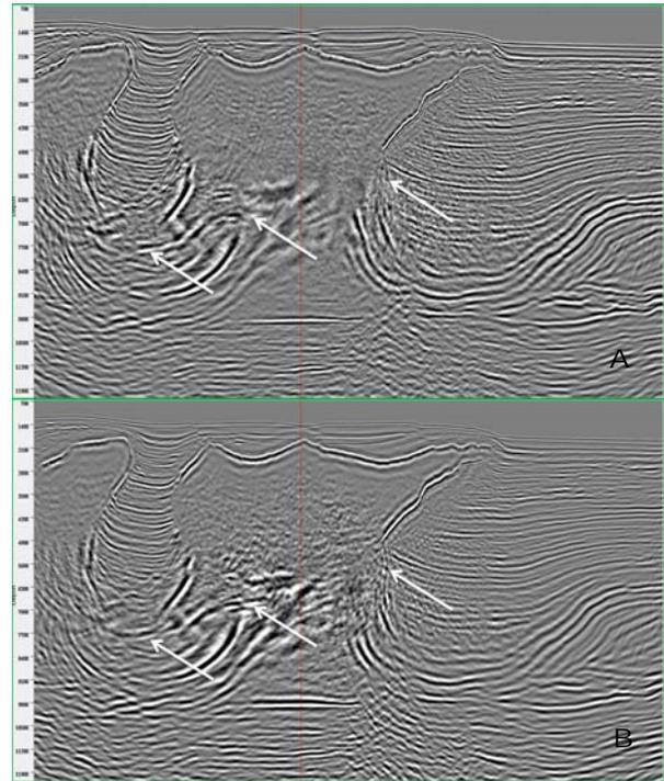
Figure 8: Comparison between the weighted sum stack of orthogonal WAZ RTM stack and the CFP RTM stack seen from the Kepler Survey direction.
