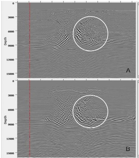
Figure 7: Comparison between the weighted sum stack of orthogonal WAZ RTM and the CFP RTM stack seen from the Kepler Survey direction.
