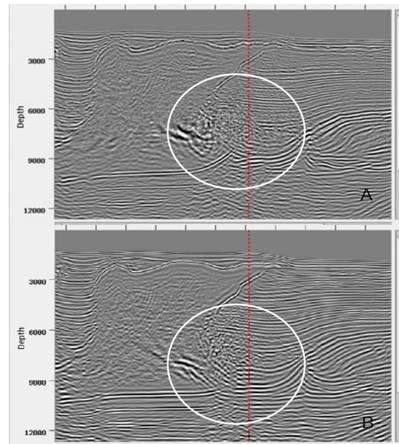
Figure 5: Comparison between the weighted sum stack of orthogonal WAZ RTM and the CFP RTM stack seen from the Justice Survey direction.
