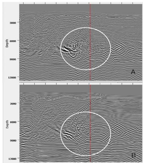
Figure 5: Comparison between the weighted sum stack of orthogonal WAZ RTM and the CFP RTM stack seen from the Justice Survey direction.
