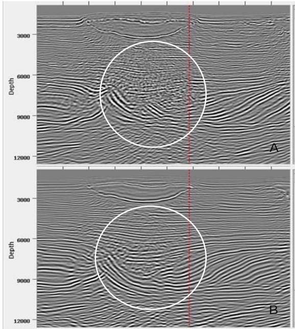
Figure 6: Comparison between the weighted sum stack of orthogonal WAZ RTM and the CFP RTM stack seen from the Kepler Survey direction.
