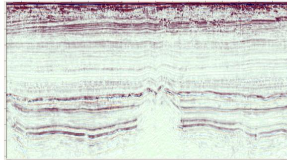
Figure 5: 2D demigrated seismic data along zigzag line
