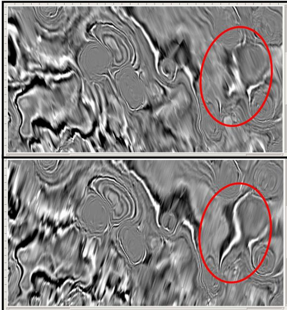
Figure 3: Examples of interpolated traces if only those traces on certain azimuthal searching orientation are used. A) along -20 degrees; B) along +20 degrees (close to the strike direction)
