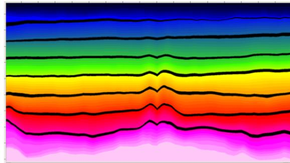
Figure 6: 2D geological time model which ties at all intersections between 2D lines. The line shown here is the same as shown in Figure 5. The Model layering closely matches the geology.
