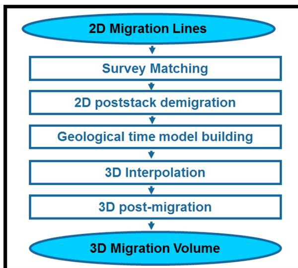
Figure 1. Work flow diagram for 2D Cube technology.
