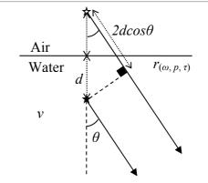
Figure 1 The time delay between a source signal and its ghost is angle dependant and uniform for a plane wave, i.e. along a slowness trace with a certain ray-parameter.
