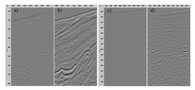
**Figure 4** A 2D profile from the West of Shetland basin with and without application of de-ghosting in the  $\tau$ -p domain, deconvolution in common-p and zero-phasing: a) and b) in a shallow zone, c) and d) in a deep zone. Note the improvement in resolution and also the enhancement achieved by exploiting the contribution from retrieved frequencies. Interpretable low-frequency signal is made available down to around 2 Hz.
