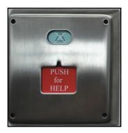
The High Security Push Button Cover Plate (R5HSPBCP) is a .050", stainless steel plate, designed to protect Rauland R5 Code (354011) and Staff Assist Station (354012) when used in psychiatric wards and other high security hospital areas. The plate installs over the push button stations without drilling or modification to the station. This plate is NOT USED with the R5KLS-4.
