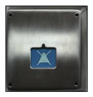
The High Security Cancel Station Cover Plate (R5HSCSCP) is a .050", stainless steel plate, designed to protect Rauland R5 Cancel Station (354010) when used in psychiatric wards and other high security hospital areas. The plate installs over the station without drilling or modification to the station. This plate is NOT USED with the R5KLS-4.
