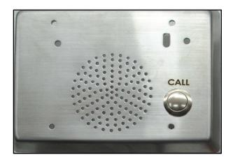
The High Security Steel Cover Plate (R5HSSCP-1) is a 3 gang, .050", stainless steel plate, designed to protect the R5 Staff Station (353101) when used in psychiatric wards and other high security hospital areas. The plate incorporates a vandal resistant dry contact switch which is used in conjunction with the R5KLS and is used to initiate a call from the room. The plate installs over the R5 Staff Station (353101) without drilling or modification to the station.
