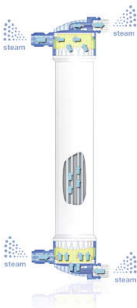
INLINE steam sterilisation process.
