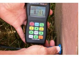
**Ultrasound Thickness Gauge** An ultrasonic thickness gauge is a nondestructive measurement tool used to accurately evaluate section loss in tubular structures.
