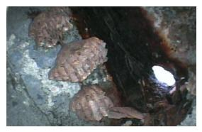
**Internal Borescope** Internal borescopes are inserted into tubular structures to identify unseen and latent corrosion that may have otherwise been undetected due to a lack of visible exterior corrosion.
