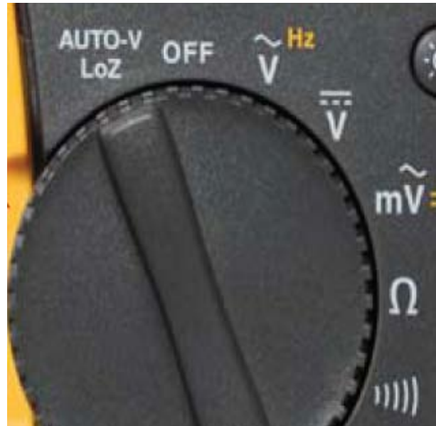
Figure 16 - Digital Voltmeter with low impedance voltage measurement option built in.
