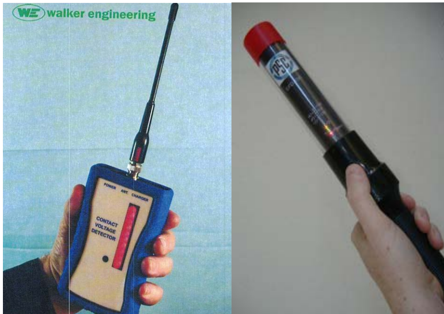
Figure 17 - Examples of a handheld electric field detectors which can be used to check ground references for voltage
