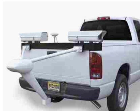
Figure 13 - SVD 2000 mobile detection system
