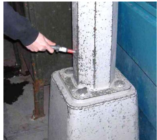
Figure 14 - HD Electric LV-S-5 Low Voltage Detector
