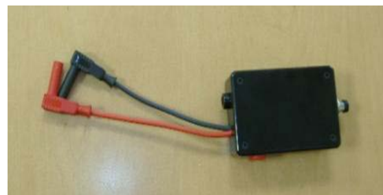
Figure 19 - Pushbutton shunt resistor puts shunt resistance in parallel with test leads only while button is engaged, allowing quick measurements with and without shunt without the need to move test leads.
