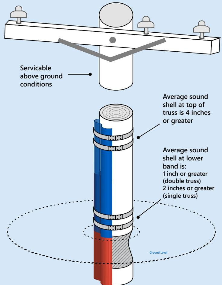
**Figure 3** Minimum Wood Pole Condition Requirements for Steel Truss Restoration
