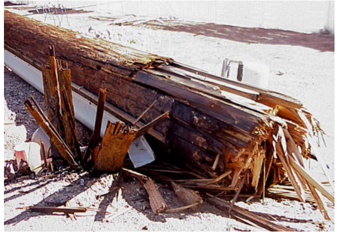
Figure 1. Wood Pole Bending Failure.
