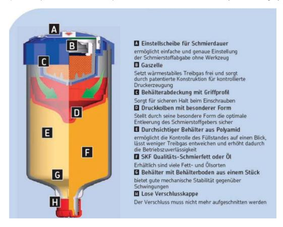
In the closed compartment the plus- minus- poles are in contact with a gel and the production of gas is activated by an electric short circuit. The amount of gas pro time unit will be regulated through an electrical resistance. The greater the resistance, the slower the production of gas. The amount of gas is proportional to the current which flows through the battery. If the supply is interrupted, the gas production will be stopped for a short period of time.
