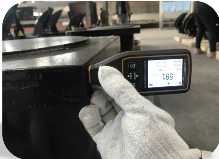
Coating Thickness Checking
