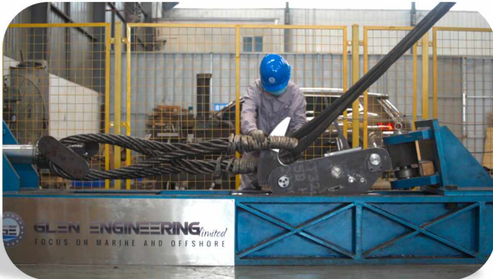
Load Test at 100% ~ 150% S.W.L.
