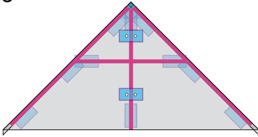
Poke holes for the top and bottom of the bridle on both sides of the spine.
