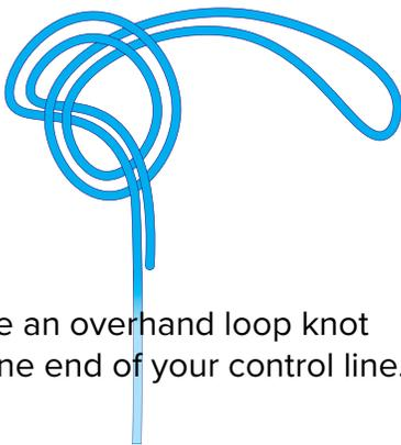
Tie an overhand loop knot at one end of your control line.
