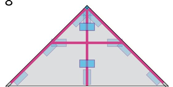
Reinforce connection points for the bridle with tape.
