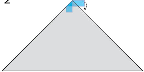
Fold tape over the top to reinforce the tip.
