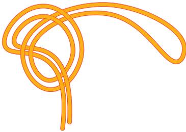
Fold an 8-inch piece of string in half, and tie an overhand loop knot at one end.
