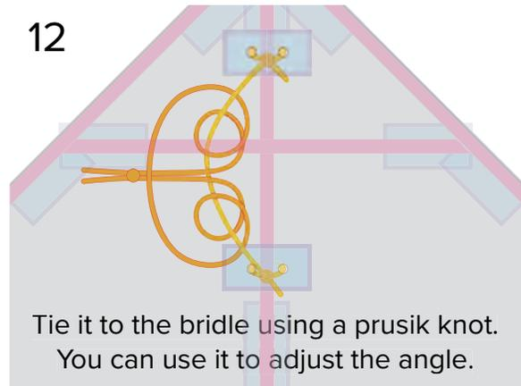
Tie it to the bridle using a prusik knot. You can use it to adjust the angle.
