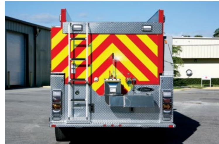
Swivel dump valve and safe access to hose bed. Shown on a commercial tanker.
