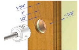
**NOTE:** In Step 2.3, if there is a gap between the drywall and the stud, measure the distance and add to the bore hole depth. Hole depth must accommodate lock barrel preparation in Step 4. You can deepen trim bore as needed after that step.
