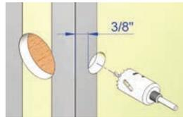
3.2) Dry Wall or Flat Casing opening; Use a 1" hole saw to cut lock bore hole to depth as shown in chart.
