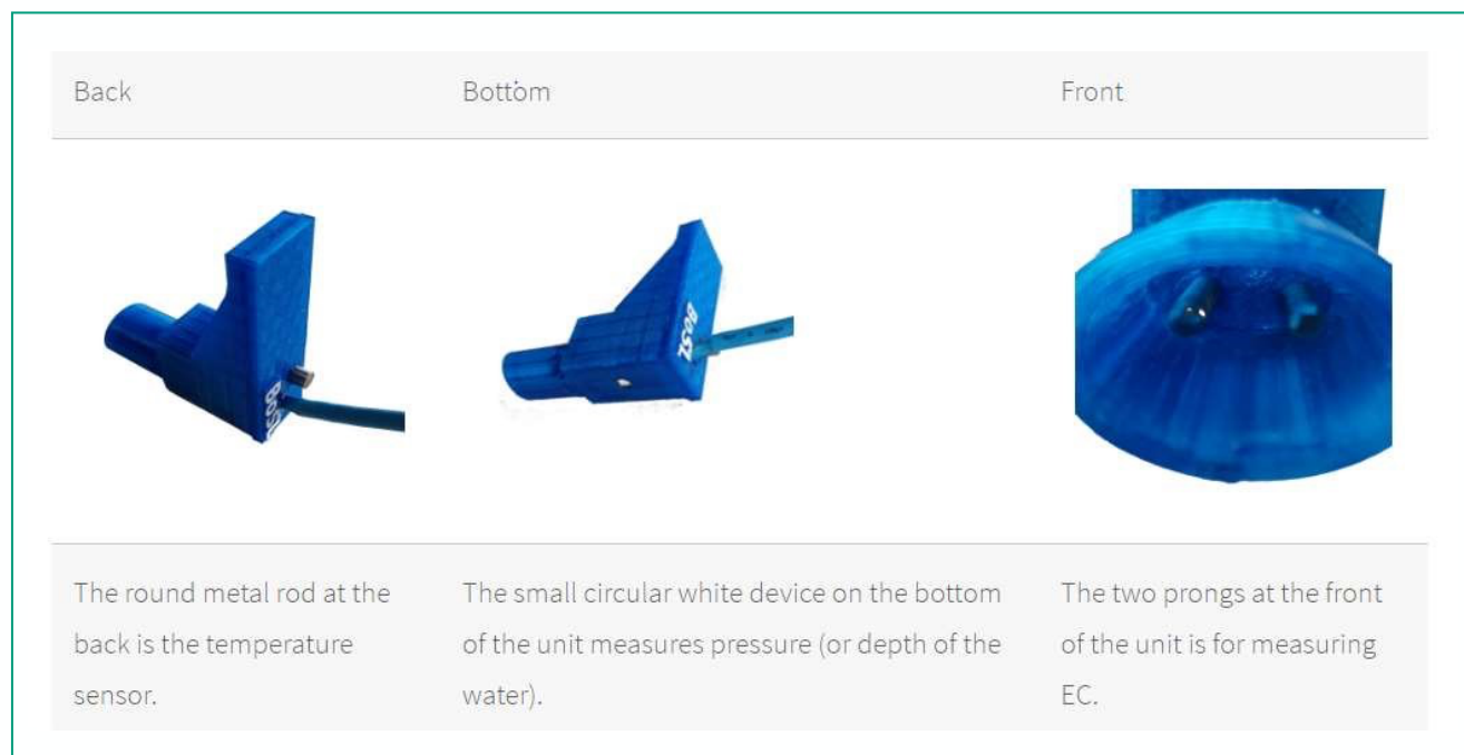
Figure 5: Future development in conjunction with Melbourne Water and Monash University highlighting the new all-in-one depth, EC and temperature probe which now has adequate shrouding on the EC sensor for more accurate measurements.
