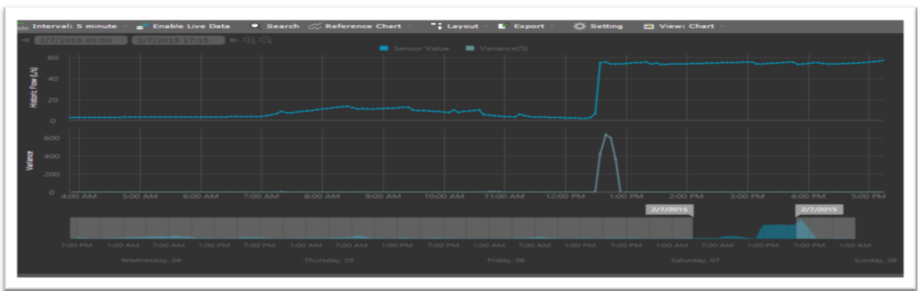
Figure 15: Burst detection using changes in the variance of SCADA data received from sensors was an effective method of detecting status changes within a water distribution network, including the detection of both leaks and bursts even within a sampled data environment.
