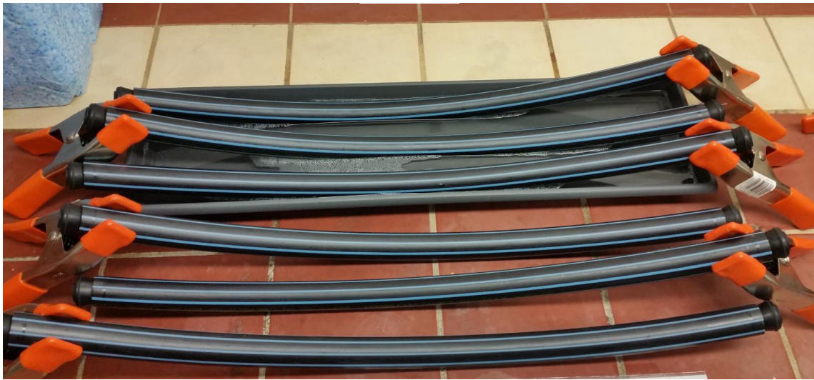
Figure 1: One of two sets of three HDPE pipes immersed in 3% AFFF (top) and three adjacent control pipes (bottom)
