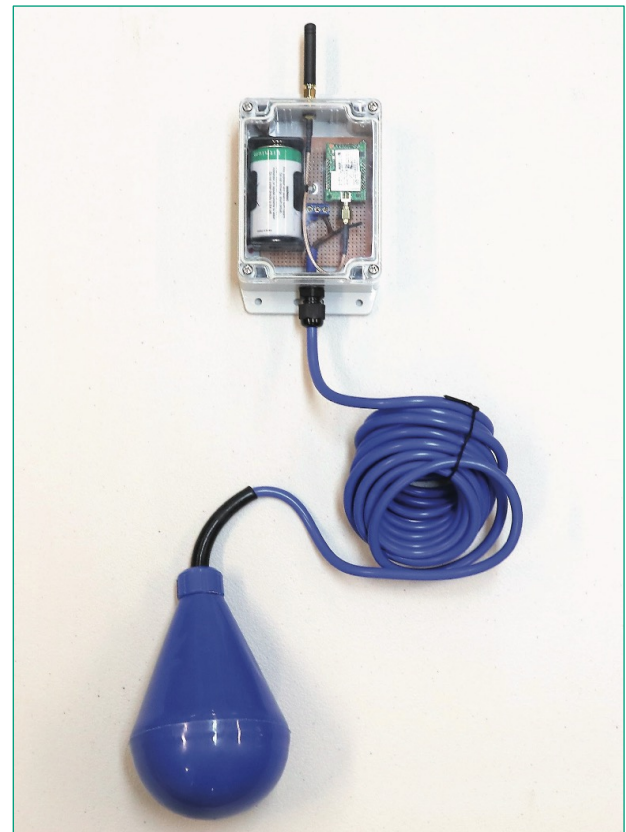
Figure 2: Sydney Water-developed and assembled IoT Sewer Level Transmitter with Float Sensor
