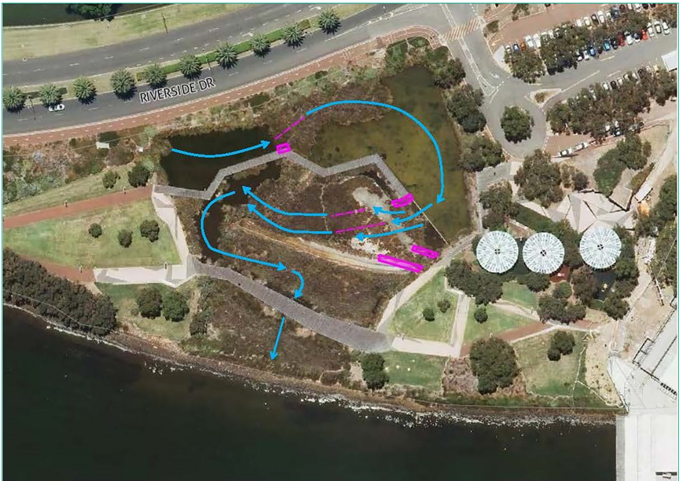
Figure 1: Point Fraser Wetland, East Perth Western Australia. Remediation design trialed under induced flow conditions at Point Fraser wetland, 29 June - 12 July 2016. Pink dashed line indicates channeling within dense vegetation, pink polygon indicates location of sandbagging and blue arrows indicate the anticipated route of water flow throughout the wetland.
